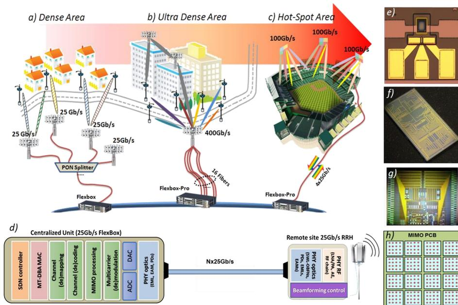
Fig. 1. a) 5G-PHOS network for PON-overlaid dense area coverage, b) Ultra-Dense areas, c) Hot-Spot case at a stadium, d) centralized Physical Layer function split approach, e) 10G InP Photodiode, f) Optical beamformer chip, g) Triplex mini-ROADM chip, h) massive MIMO antenna PCB.
