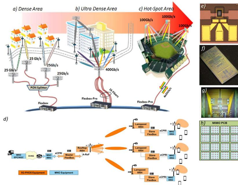
Fig. 1. a) 5G-PHOS network for PON-overlaid dense area coverage, b) Ultra-Dense areas, c) Hot-Spot case at a stadium, d) centralized analog fronthaul architecture, e) 10G InP Photodiode, f) Optical beamformer chip, g) Triplex mini-ROADM chip, h) massive MIMO antenna PCB.
